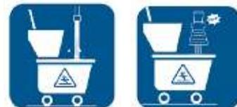
Fill Bucket > Hold Activator Above Bucket > Twist CAP On (3X)
